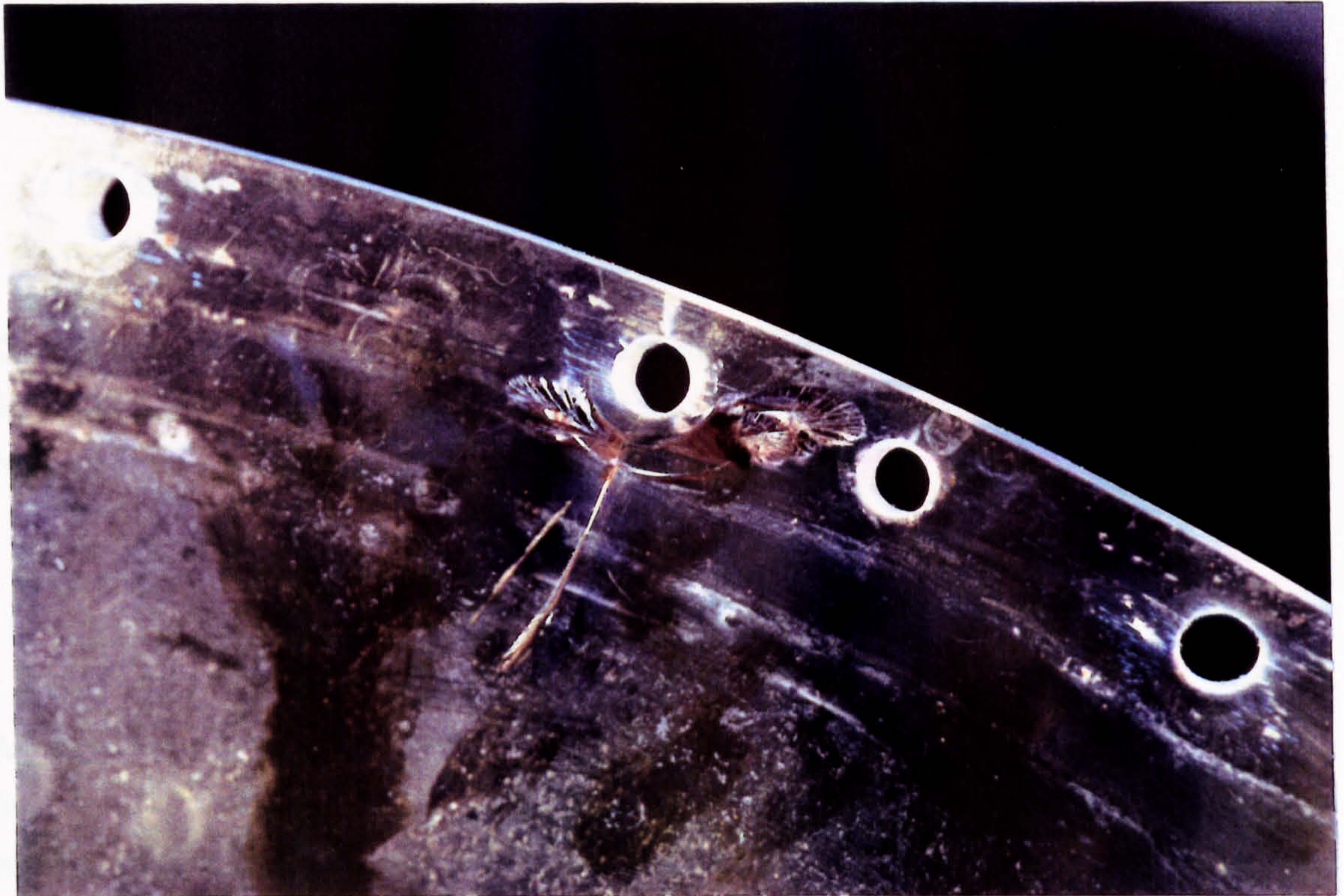
Photograph (c) : Stress Fractures produced on the Polycarbonate Window
