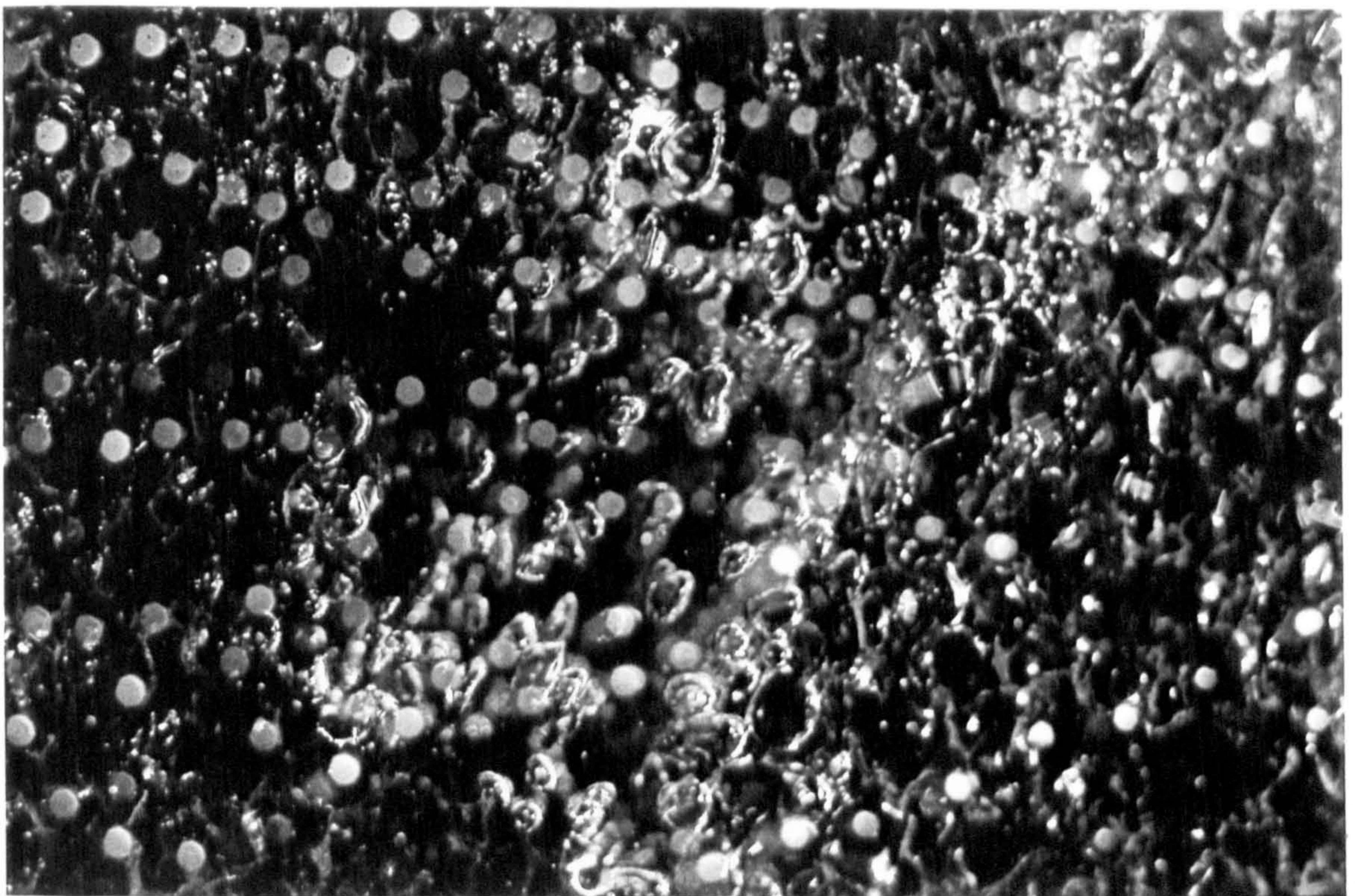
Photograph No.16 : Window 12 : Gas - Liquid Interface Speed 200 rpm, Liquid Flow 0.1 l/sec, Gas Flow (stp) 1.0 l/sec
