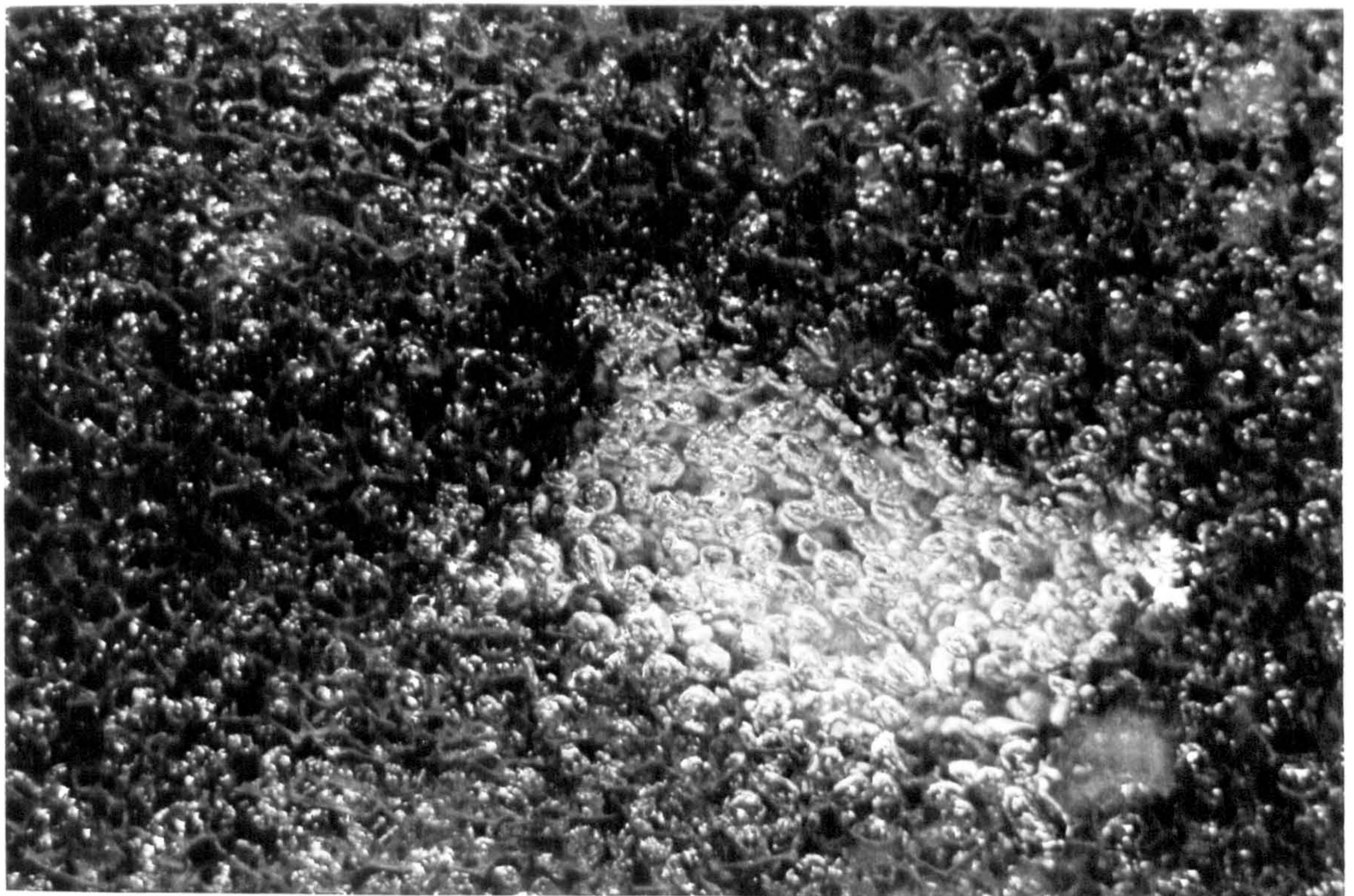
Photograph No.20 : Window 12 : Modified Gas Nozzles Speed 250 rpm, Liquid Flow 0.1 l/sec, Gas Flow (stp) 1.1 l/sec
