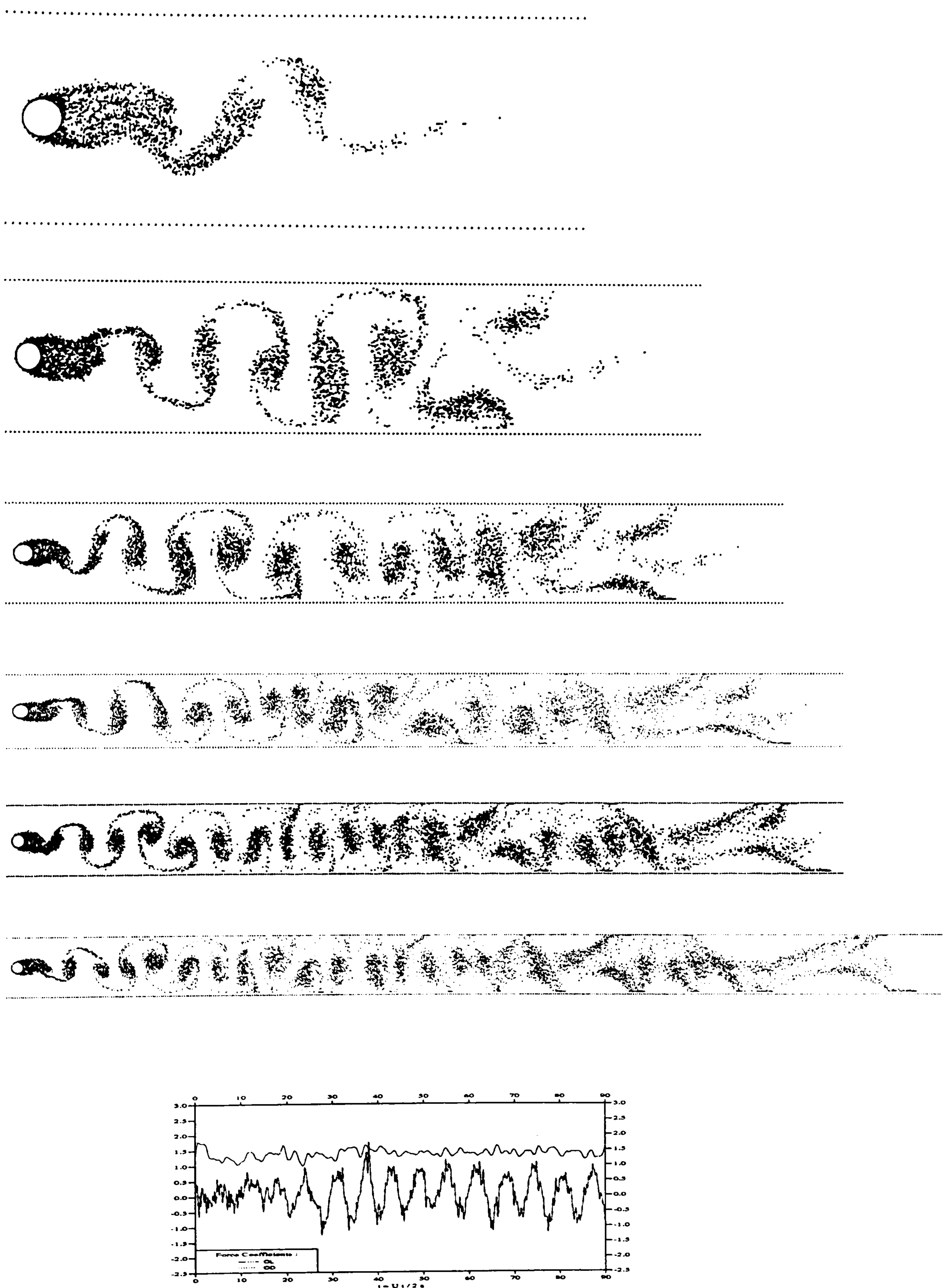
Figure D.2.- Flow Pattern at t = 10, 20, 30, 40, G/D = 6 , and the Force Coefficients for Re = 1000
