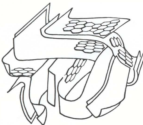
Figure 1.15 A schematic structure of activated carbon
